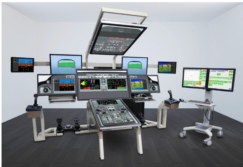
Fig. 7. The Aircraft Cockpit Universal Prototyping Bench of GosNIAS
